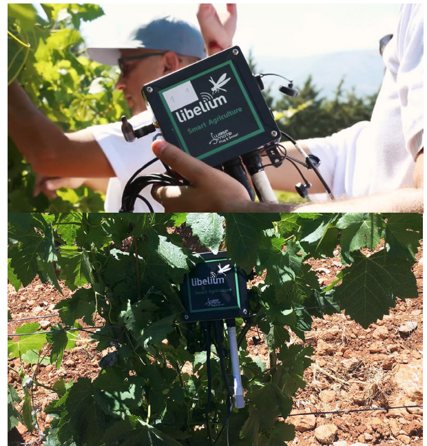
Wasmote Plug & Sense! Smart Agriculture PRO positioned at the vine trunk
