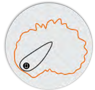
Figure 5. R350 5GHz Elevation Antenna Patterns
