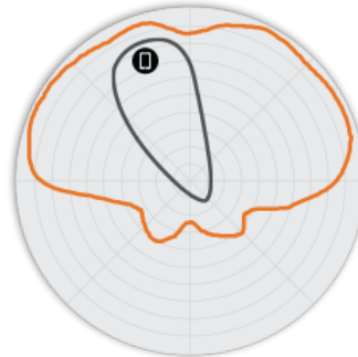
Figure 4. R750 2.4GHz Elevation Antenna Patterns
