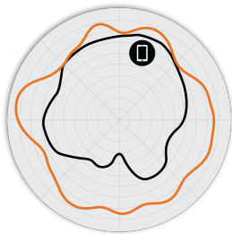
Figure 2. R760 2.4GHz Azimuth Antenna Patterns
