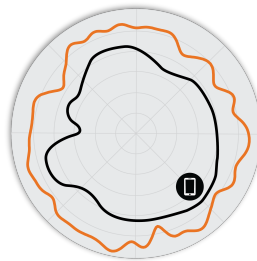
Figure 3. R760 5GHz Azimuth Antenna Patterns
