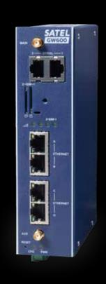
The versatile 2G/3G/LTE wireless router is suitable for a variety of industrial deployments. The compact structure makes it excellent for M2M applications like SCADA, telemetry and intelligent traffic systems. The router supports the following radio access technologies: LTE, HSPA+, HSPA, UMTS, EDGE, GPRS and GSM.
