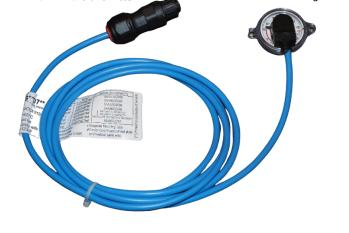
Many existing domestic storage tanks are equipped with weak drive magnets suited for low friction directindicating dial assemblies. As the Hall Effect Twinsite is a contactless sensor it can be utilized for a retrofit on these vessels to provide an electrical output which can be used for remote indication of tank levels.
