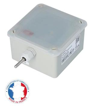
The **Outdoor Temperature Sensor** can be used to remotely monitor the outdoor temperature in order to provide climate data, to measure the temperature inside a room in a positive or negative cold temperature environment. Data transmission over the public or private LoRaWAN® network is done periodically or immediately in the event of an alert when the minimum or maximum temperature threshold is exceeded.
